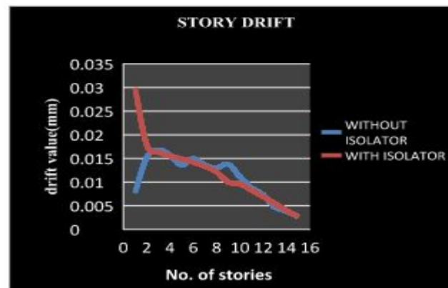
Fig.14.storey drifts of fifteen storied building.
